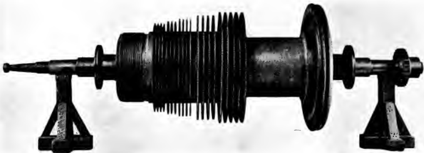
Fig. 7. View of low pressure turbine sprindile showing ahead reaction blading, astern impulse wheel, water gland runners, and flexible coupling (right).
